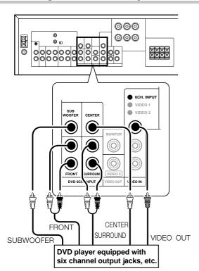
The sound input to DVD 6CH. INPUT is paired with the video signal input to 6CH. INPUT.
